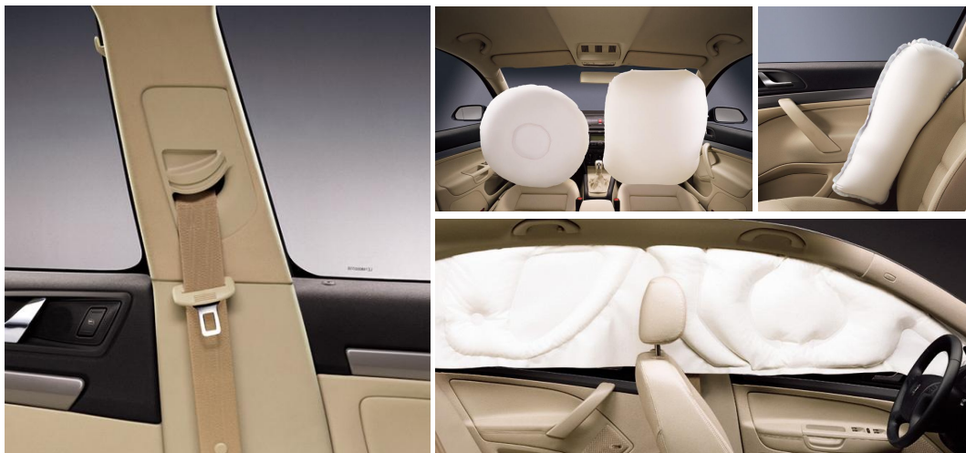
Examples of Octavia passive safety elements: Seat belts, driver and front passenger airbags, side and head airbags
