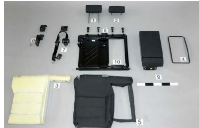
Disassembly study - example of the disassembly of the front door and rear seat backrest of new Octavia
