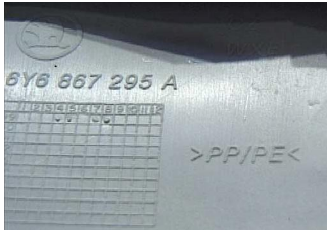
Example of part markings (upper trim of the C-pillar - Fabia)
