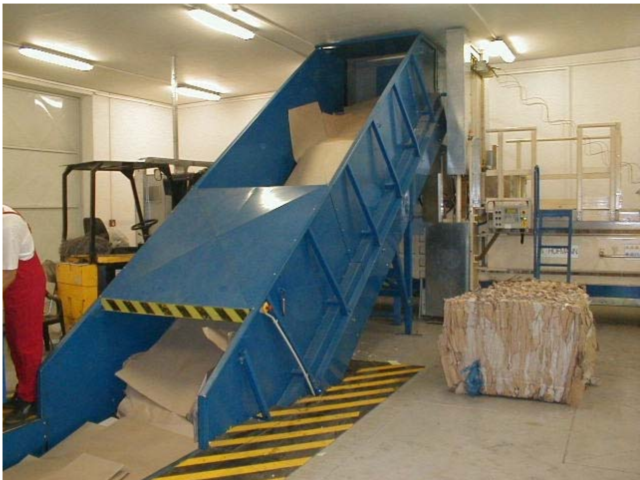
COMPACT NO 60 - automatic horizontal press for waste packaging
